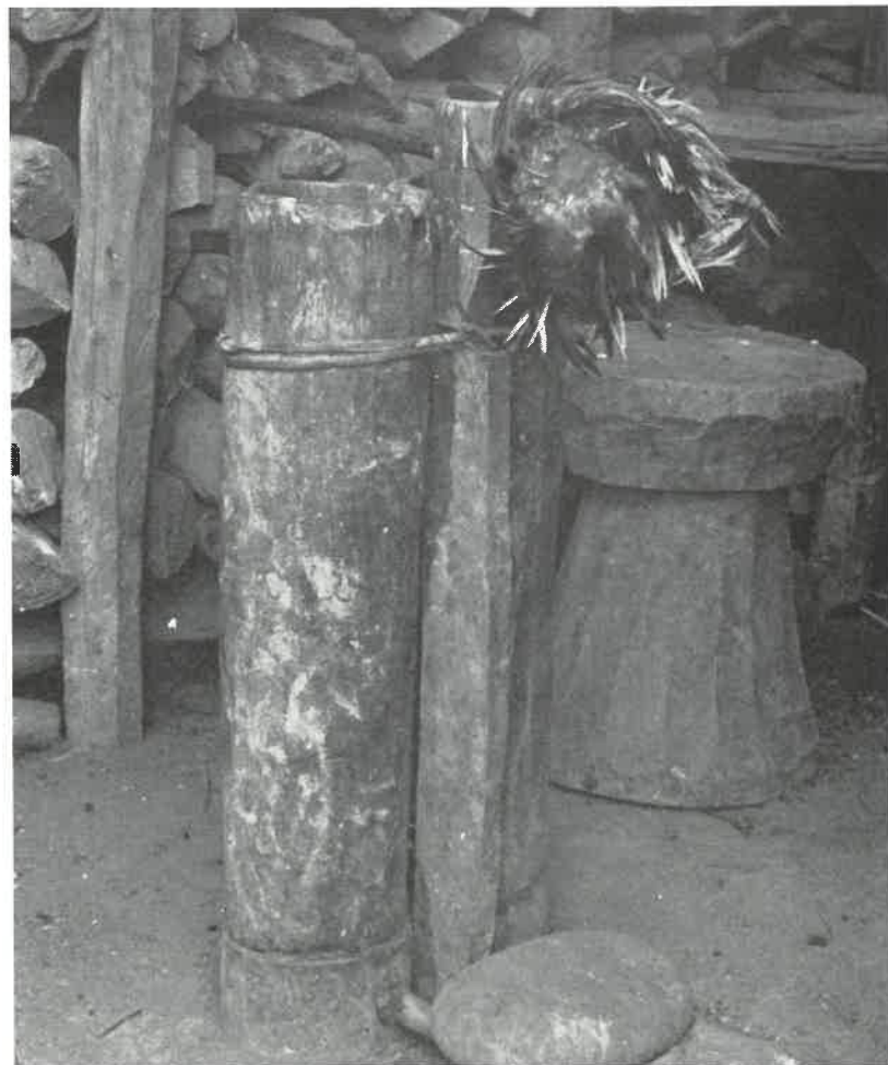
Fig. 26. Hnaring blacksmith's "Malayan" piston bellows forge.
